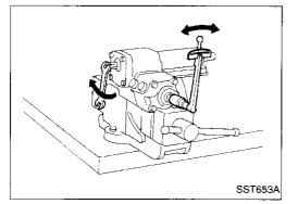
b. Turn stub shaft all the way to right and left several times.c. Measure turning torque at 360° position from straight-ahead
